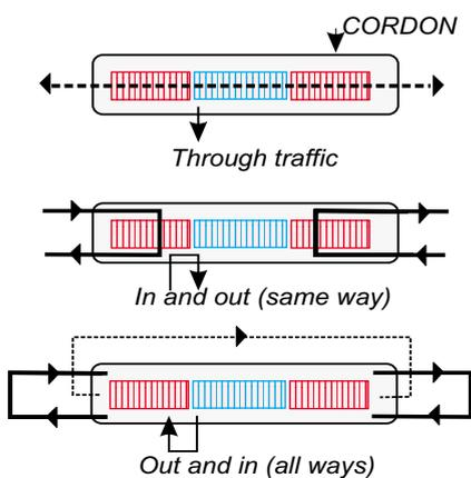
Fig 2.6 The cordon should be established outside the transition zone. Traffic volumes should be measured at points where the road crosses the cordon.
