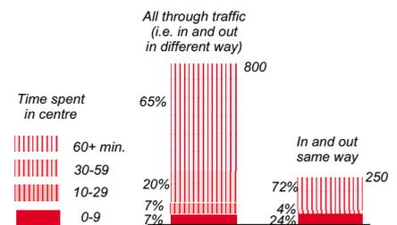
Fig 2.8 An example of the results of a number plate survey. A number plate survey at the cordon points enables non-stopping through traffic to be determined. It also provides information on non-stopping heavy vehicles.
