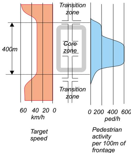
Fig 4.13 Determining speed and activity profiles
