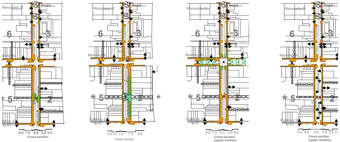
*Option A* This is a least cost option. The focus is at the mid-block crossing. There is a narrow median and much of the existing pavement can be re-used.
