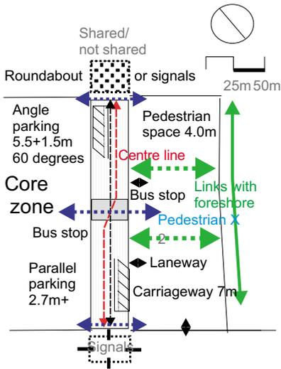
Fig.4.12 Example of parameters for concept design
