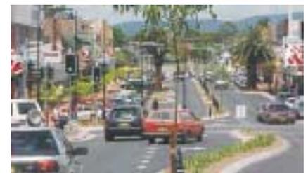
Fig 4.16 Provision for turning movement increases pedestrian crossing distance and requires space for waiting vehicles (Taree).
