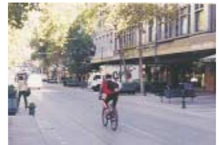
Fig. 4-8 In a low speed environment cyclists can share the carriageway, provided vehicle traffic volumes are not high.
