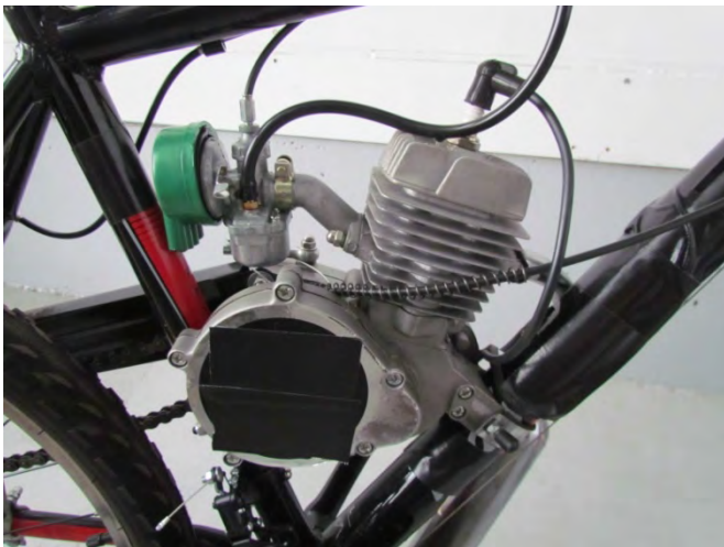
Figure 11: Motor Setup for 48cc bicycle Note the exposed engine and components, including fuel lines
