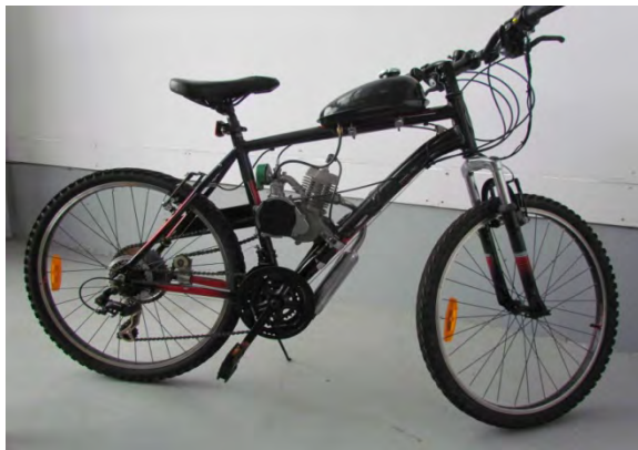
Figure 3: 48cc unrestricted petrol-powered bicycle
