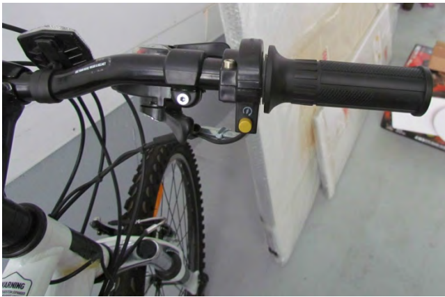
Figure 9: Right hand controls, 48cc bicycles Note: The grip has been modified as a throttle.
