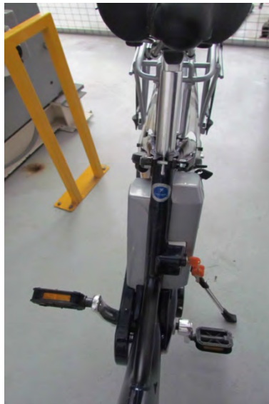
Figure 17: Pedalec's motor and battery integrated unit
