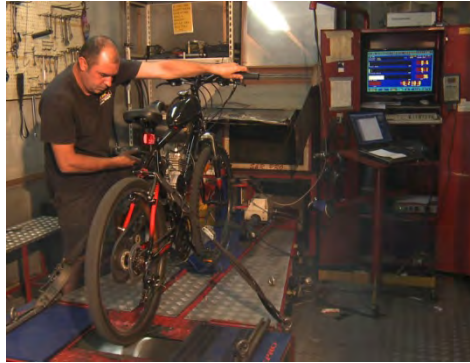
Figure 16: Dynamometer Test Setup with 48cc unrestricted petrol-powered bicycle
