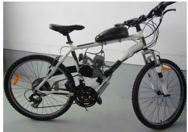
Figure 2: 48cc restricted petrol-powered bicycle
