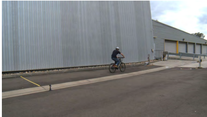
Figure 15: Braking Test Setup Note yellow braking line
