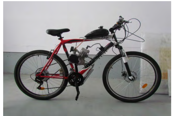
Figure 4: 66cc petrol-powered bicycle
