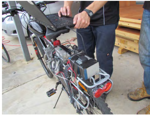
Figure 13: Data Acquisition Setup for Acceleration Tests Note: The device is fitted to one of the 48cc petrol-powered bicycles and is connected to a laptop computer for calibration.
